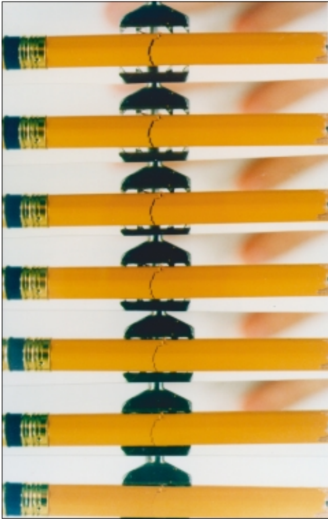
Figure 5) The teeth are just barely penetrating the fractured pencil in the photograph on the top of this time-lapsed photograph figure. As the teeth penetrate progressively deeper to the bottom of the figure, the teeth have penetrated completely and the pencil fracture gap is eliminated
