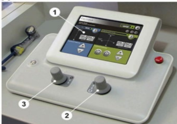
Figure 2(A) Representative picture of the control console: 1- touch screencontrols; 2- guidewire joystick; 3- balloon/stent catheter joystick
