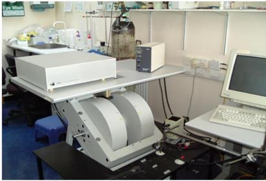
Figure 1(A, B) A Diagrammatic 2-D representation of the gold-plated ESR cavity and grid onto which the 1 cm 2 laser beam was directed. It was established by eye that the beam was incident upon the dark-brown hair strands (10 mg) contained vertically in a 50 µl silica capillary tube (width 1.4 mm) within the ESR cavity of the Bruker EMX Spectrometer (B)
