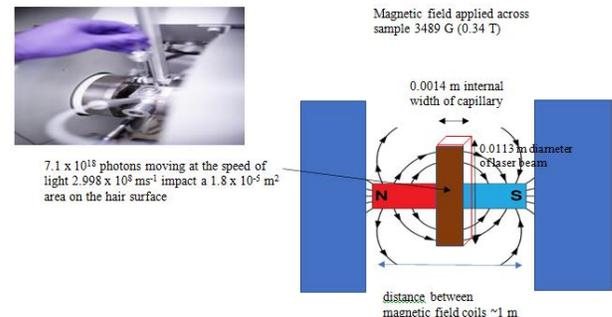
**Figure 7**) Derivation of a simplified equation from the Biot-Savart Law which describes the magnetic field due to a moving charge for the laser pulse impacting hair at the centre of the ESR cavity. Inset photo shows how a sample is inserted between magnetic field coils in an ESR spectrometer (here Jeol spectrometer)
