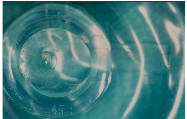
Figure 6) In three of the implants with delayed leakage (Table 1), fibrous tissue was observed in the valve mechanism. This may have served as a 'wick' to stimulate fluid leakage
