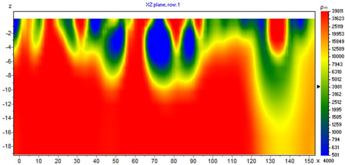
Figure 9) Volume Slice of the outmost profile or section along the x-direction after noise filtering.
