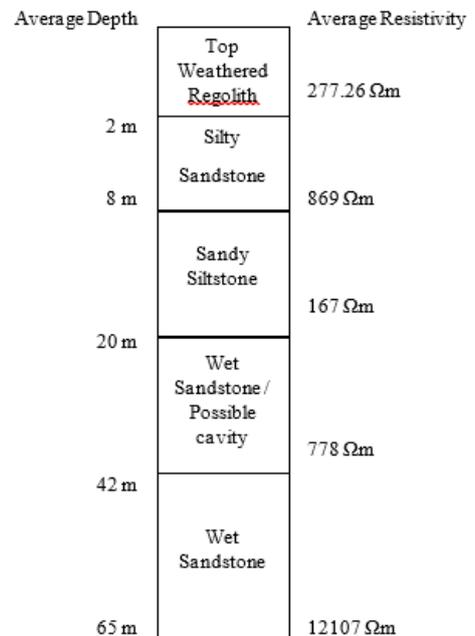
Figure 8) Pseudo-section of the electrical resistivity distribution at ves location 2.
