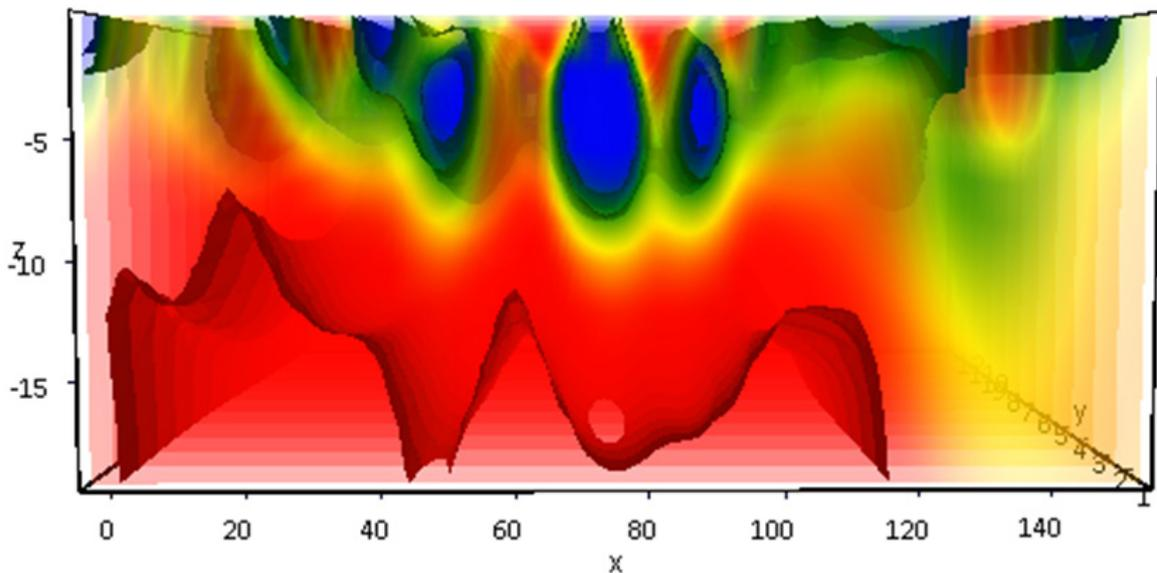
Figure 11) Volume slice of the outmost profile or section along the x-direction with derived isosurfaces enhanced for better visualization of the cave geometry.
