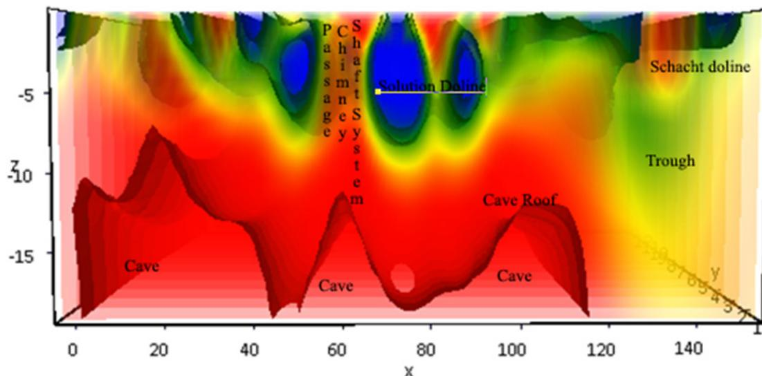
Figure 12) Volume slice of the outmost profile or section along the x-direction with derived isosurfaces and interpretation of the features seen on the image.
