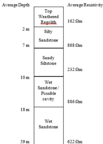
Figure 7) Pseudo-section of the electrical resistivity distribution at ves location 1.
