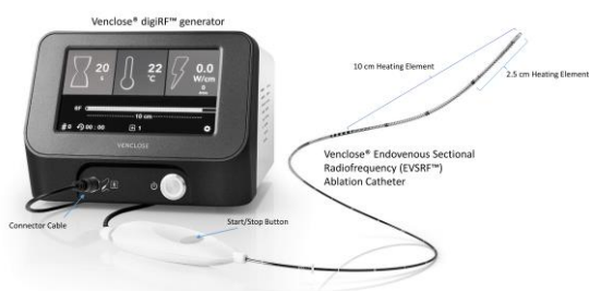
Figure 1) The Venclose Endovenous Sectional Radiofrequency Ablation System (Venclose/Becton, Dickinson and Company, USA) is a two-piece system consisting of a of Radiofrequency generator and a 6 F ablation catheter with two heating element lengths (2.5 cm and 10 cm) to thermally ablate a superficial refluxing vein
