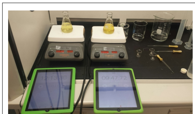
Figure 1 Silver nanoparticle fabrication by silver nitrate dissociation.
