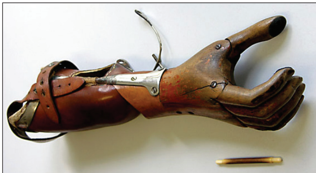
Figure 5) Sauerbruch's prosthetic hand design in the early 20th century gave many amputees a high degree of functional independence. Video captures of patients using the prosthesis to perform various activities may be viewed at http://vlp.mpiwg-berlin.mpg.de/library/data/lit38416 . Image credit: Hermann von Helmholtz Center for Cultural Technology, Humboldt University of Berlin < http://www.sammlungen.hu-berlin.de/objekt-des-monats/2005/11/ >
