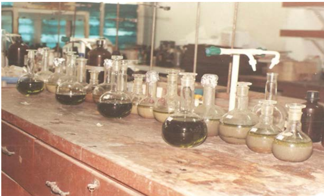
Figure 2b) Crude Extracts from Galatea paradoxa in the laboratory for PCBs analysis
